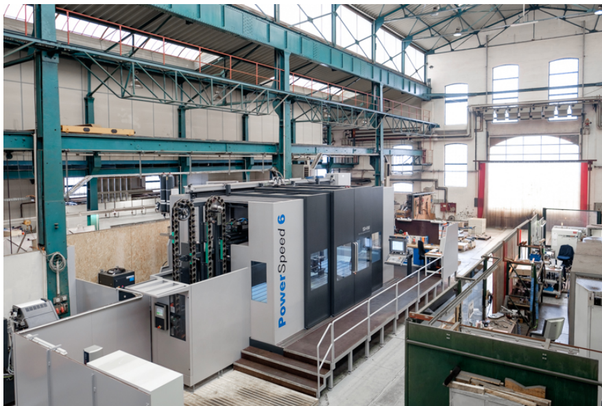
Image no. 17-02 SHW_MNR-PS6.jpg Montagebau-Neptun Rostock uses the new flexibility it has gained from the PowerSpeed 6 by SHW Werkzeugmaschinen for its production of large-sized parts and assemblies for shipbuilding, machine construction, the petrochemical industry and the offshore wind energy sector.
